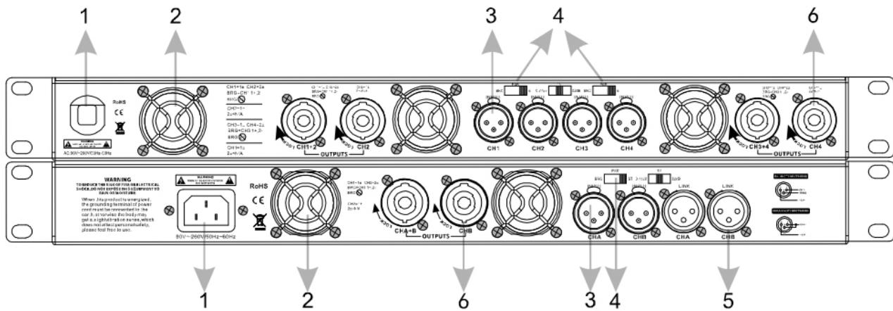
top: larger models with locking mains inlet, bottom: smaller models with IEC inlet
